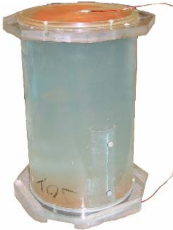
Fig. 3. A cylinder shaped phantom in which the bases are two copper plate electrodes. The cylinder is filled with water containing \text{CuSO}_4 and \text{NaCl} . Externally applied current is injected through the top electrode and leaves at the bottom one.
